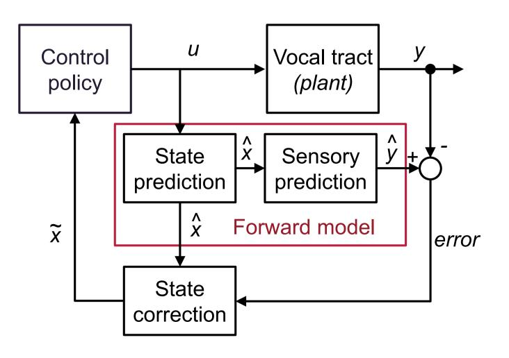
A simplified state-feedback controller. The lower-level (articulatory) controller in FACTS has this structure.
