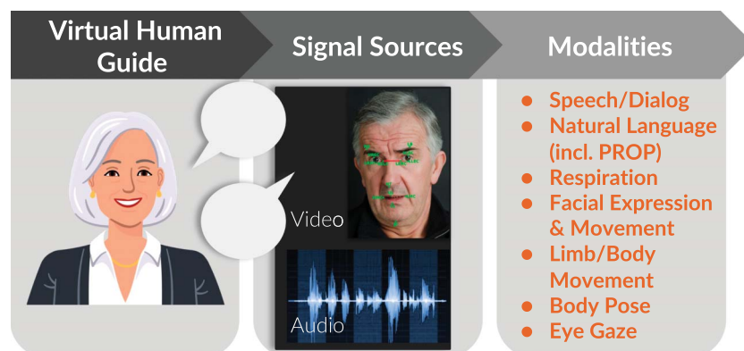
Figure 2. The Modality multimodal dialog platform for remote patient assessment uses a virtual human guide, Tina, to engage participants in an interactive conversation, record their audio and video signals, and extract multiple modalities of health information therefrom. PROP = Patient Report Of Problems.
